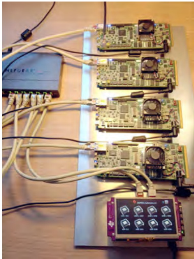
Fig. 13 Experimental hardware setup ‘ARM setup’ reflecting a fully customized embedded board. The experiments are based on Ethernet and an additional prediction is calculated on how a PCIe based custom circuit board would behave.
